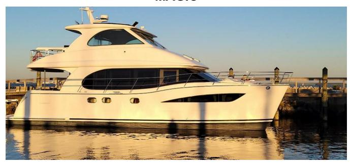
LOA:52' (15.85m)Beam:22' (6.71m)Max Draft:4' 9" (1.42m)Clearance:25' (7.62m)
